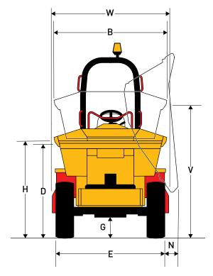
Load-over height: Skip down - 1395 mm Skip up - 2000 mm
