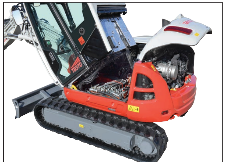
Tilt-Up Cabin Delivering Excellent Serviceability
