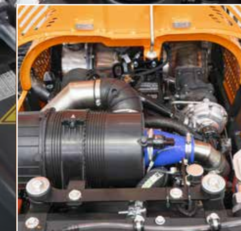
MOTORE YANMAR DA 60 CV STAGE V YANMAR ENGINE 60 HP STAGE V
